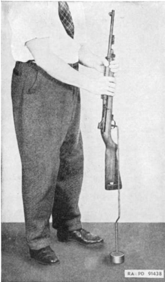
Figure 10. Testing Trigger pull.
